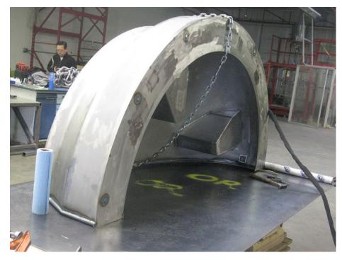
One-half of Lower Head. Note Support Legs inside of the Structure
