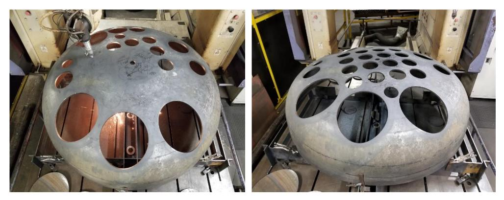
Laser machining of the penetrations to attach CRD nozzles
