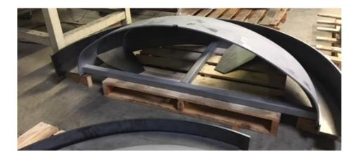
3/8-inch (9.5mm) thick lower head construction; ~70-inches (1780mm) diameter (2/3rds scale)
