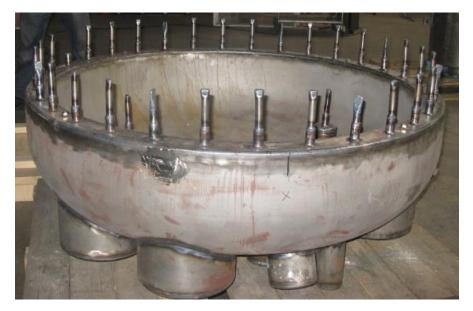
Following Degassing, All Fill Stems are Crimped and Welded Shut. Now Ready for HIP
