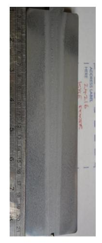
200mm Electron Beam Weld
