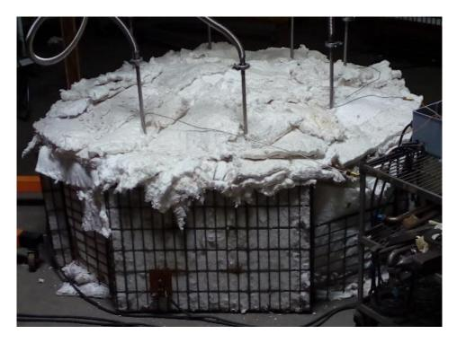
Hot Degassing of Powder Filled Upper Head
