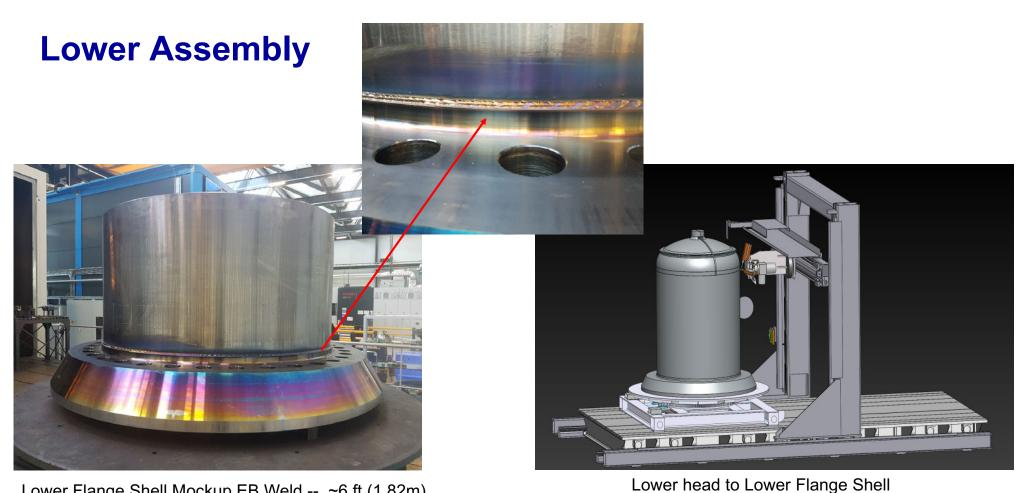
Lower Flange Shell Mockup EB Weld -- ~6 ft (1.82m) diameter (Note, mockup is upside down)
