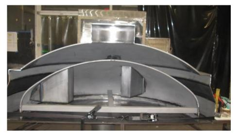
Note: Two reactor internals support structures are included for each RPV head half
