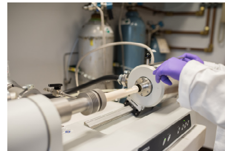
Dilatometer Liquid density measurements
