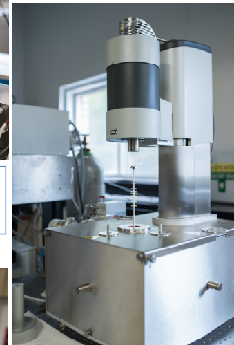
Laser Flash (LFA) Thermal diffusivity measurements
