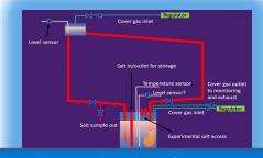
Fluoride Molten Salt Test Loop
