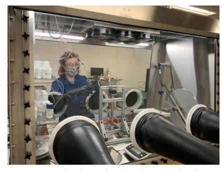
Commissioned glovebox train for experiments with irradiated materials and beryllium containing salts. The train is equipped with a deep well and an oil-free pump, which can be helpful for hydrogen and tritium experiments.
