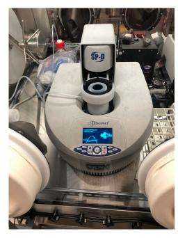
CEM Microwave digester in the glovebox train. The digester will help correlate redox measurements to elemental analysis of salt samples from the loop
