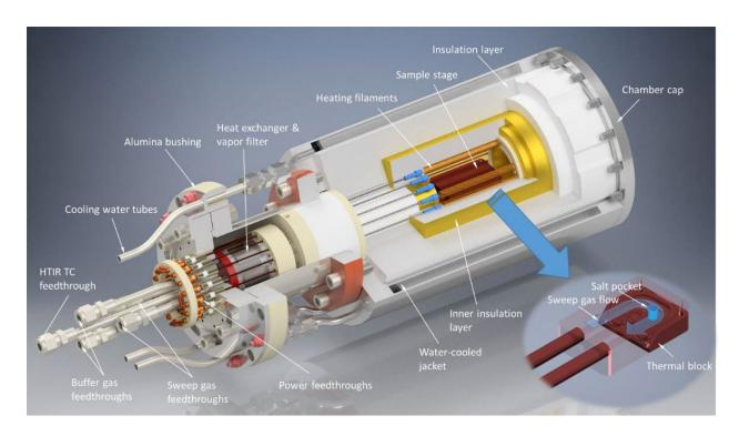
Conceptual design of the fission gas and tritium measurement irradiation chamber
