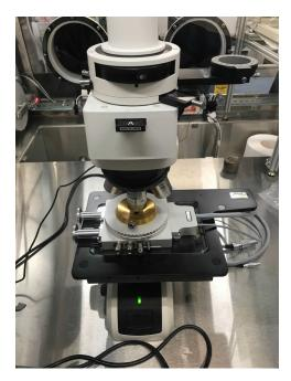
High temperature stage for electrochemistry and spectroscopy, mounted on polarized light microscope
