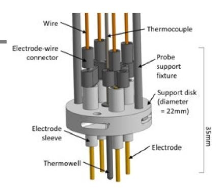
Thin film sensor for high-throughput electrochemical experimentation
