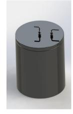
Graphite container with CVD SiC coating on inner and outer surface, ~5kg FLiNaK/batch Vendor: Ibiden USA
