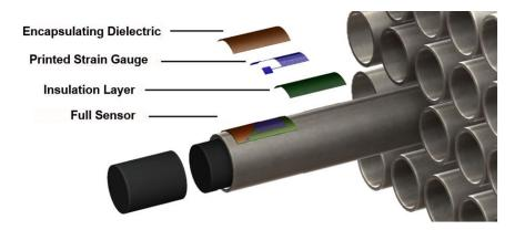
Printed strain gauge design (ASI)
