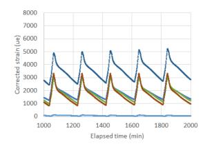
Mechanical strain histories: (L) at the start of the test, (R) around 2021-9-7
