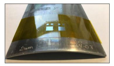
Advanced Manufactured thin film strain gauge on curved ATR fuel plate
