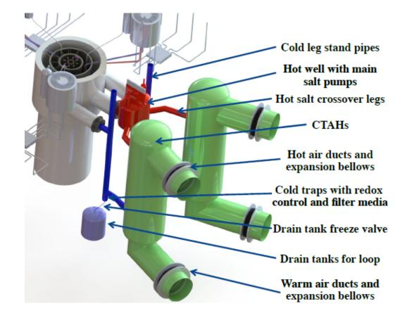
Mk1 PB-FHR, (L) Reactor vessel and cavity, (R) Heat transport system Ref: Mark-1 PB-FHR Technical Description, UCBTH-14-002, 2014
