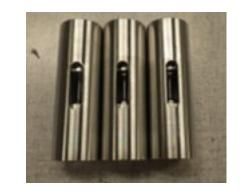
Machine inner specimen from welded rod, machine casing from larger diameter cylindrical stock
