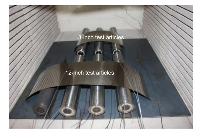
Test articles (small and large) in box furnace
