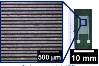
Strain gauge printed at BSU
