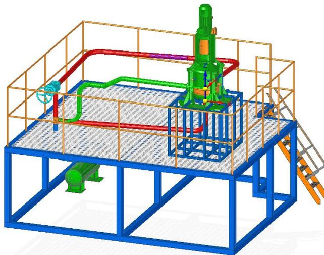
Salt pump test bench
