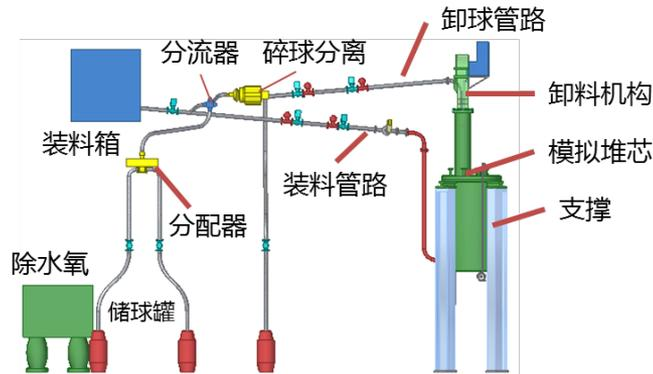
Fueling, defueling and pebble circulating simulation in molten salt condition.
