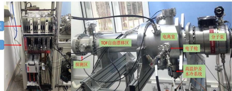
Experimental facility for study molecular and cluster structure of salt vapour.
