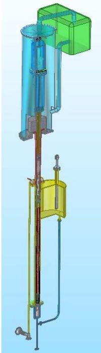
Control rod test bench. Simulate design and service condition in TMSR-SF1
