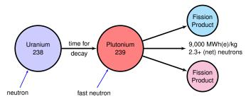
Using fast neutrons improves the performance of the uranium fuel cycle sufficiently to allow sustained further conversion and fission reactions. This has been the basis of global interest in fast-spectrum reactors for nearly 70 years.
