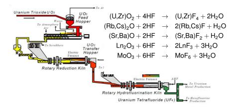
Next the powdered fuel is reduced with hydrogen and hydro-fluorinated to replace all oxides with fluorides. The constituent materials change from oxides (ceramics) to fluorides (salts) as oxygen in the spent fuel is removed as water vapor.
