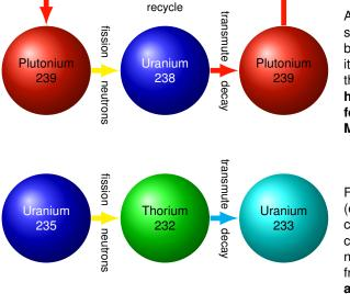
A chloride MSR (fast spectrum) could breed more fuel than it consumes, using the U-Pu cycle. This has been proposed for fast chloride MSRs.
