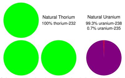
Only a small fraction of natural uranium is fissile. Most uranium and all thorium is "fertile" and can be converted to fissile material through neutron absorption.
