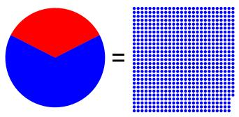
Uranium can be a sustainable fuel in a fast reactor, but using fast neutrons comes at a substantial price. Neutron cross-sections are much smaller for fast neutrons than for thermal (slowed-down) neutrons. To a thermal neutron, one atom of plutonium-239 is the equivalent of nearly 700 atoms of plutonium-239 to a fast neutron. This is why thermal reactors have a far lower fuel inventory than fast reactors, and why almost every reactor in the world today is a thermal reactor.
