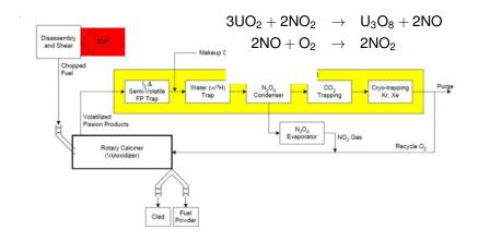
Spent nuclear fuel is first oxidized with nitrogen dioxide which causes it to pulverize into a fine powder. Xenon, krypton, tritium, iodine, and CO2 are removed as gases and purified and separated.
