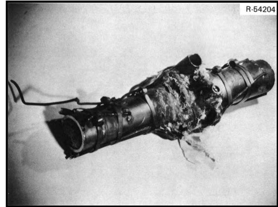
Bottom of cracked freeze valve
