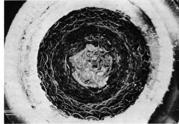
MSRE Mark 1 Offgas Particle Trap WG 67-4764
