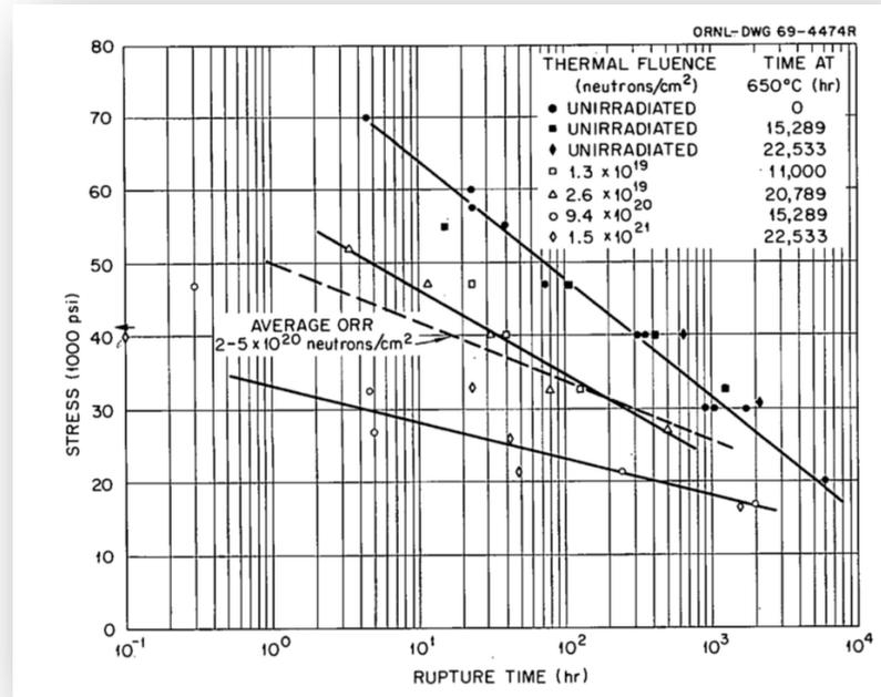
Stress rupture properties of MSRE surveillance specimens
