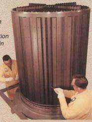
The completed reactor vessel during inspection and before installation in its containment cell. Holes near the vessel's top distributed incoming salt evenly around the vessel in a downward flow. Fully loaded, the MSRE used 11,260 pounds of a fuel salt mixture comprising lithium, beryllium, zirconium, and uranium fluoride. The coolant salt contained 15,300 pounds of lithium and beryllium fluorides.
