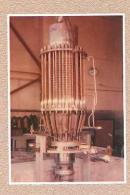
The fuel pump circulated fuel at 1,200 gallons per minute inside the MSRE reactor, which operated until December 1969.
