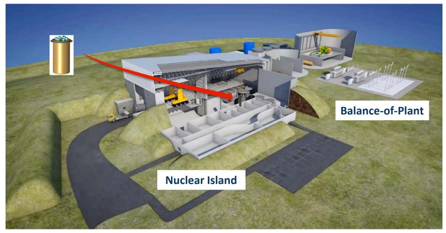
IMSR™ Nuclear Island produces 600°C industrial heat. Balance-of-Plant can be a broad range of industrial applications – not just power provision
