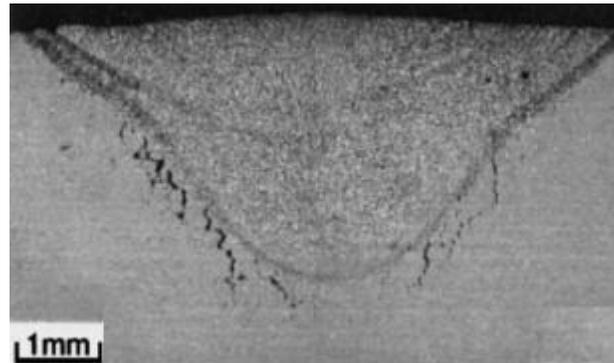
Helium-induced cracks in the HAZ after welding stainless steel contains 8.3 appm He.<sup>1</sup>
