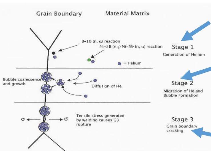
Helium generated in reactor internals throughout the life of the plant, from the boron and nickel transmutations
