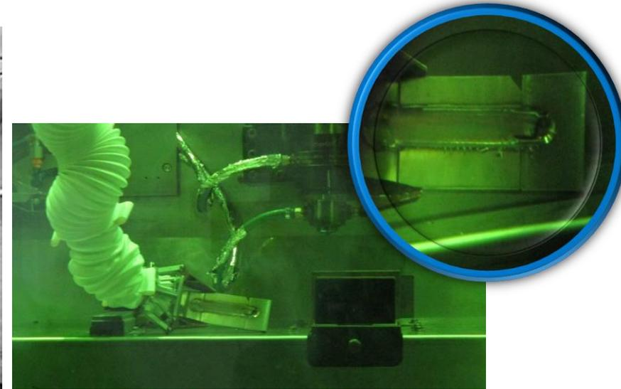
***The hot cell welding facility is a strategic asset for researchers and industry stakeholders in the development and testing of advanced weld repair technologies for extending the lives of aging reactors.***
