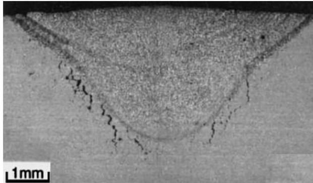
Helium induced cracks in the weld HAZ on stainless steel contains 8.3 appm He (Kyoichi Asano, et al. *Journal of Nuclear Materials*, 264, 1 – 9 (1999))
