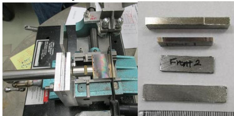
*Cutting process and sliced specimens*
