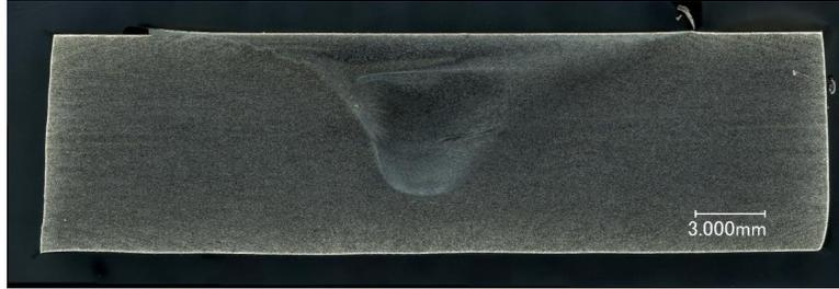
Friction stir weld on un-irradiated 304 SS
