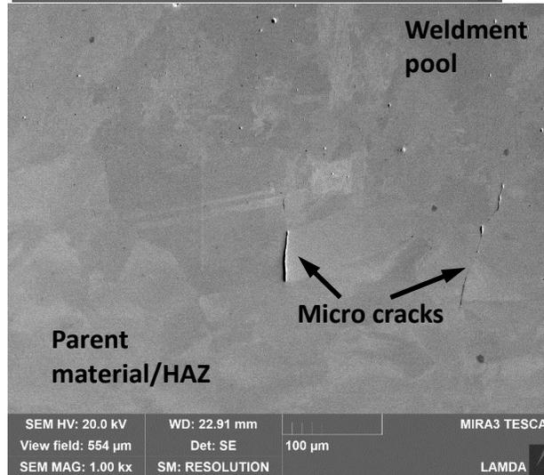
Group of minor cracks observed at the boundary between weldment and HAZ.
