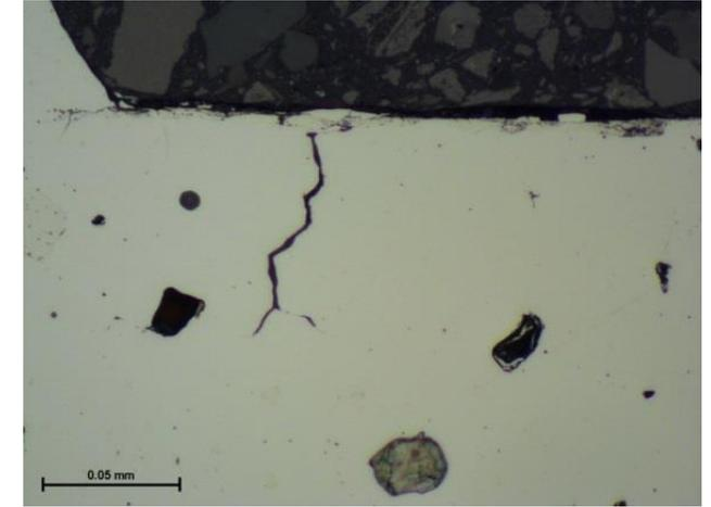
*Huge voids and cracks with fusion welding*
