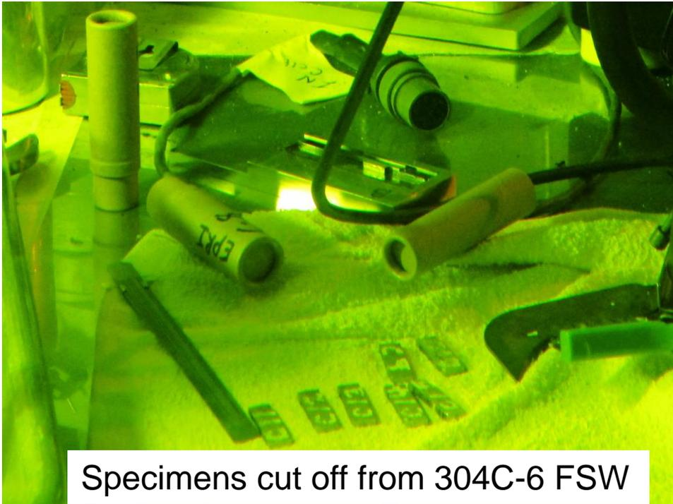
Specimens cut off from 304C-6 FSW
