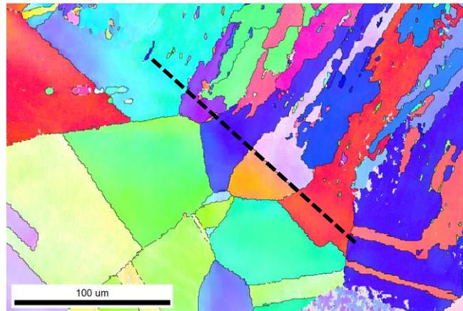
EBSD inverse pole figure around weld fusion line
