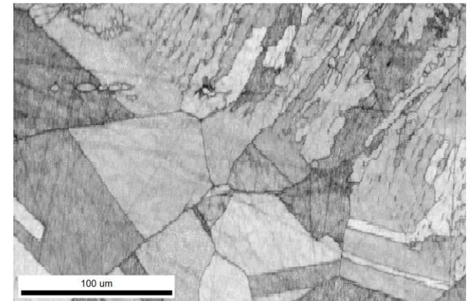
Grain around weld fusion line
