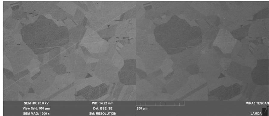
Helium induced cracks in the weld HAZ on stainless steel contains 8.3 appm He
