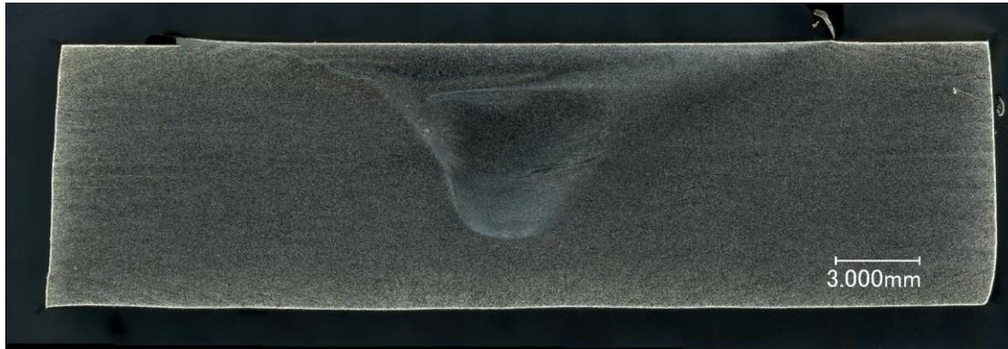
Un-irradiated 304L friction stir weld cross section
