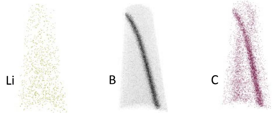
Reconstructed APT datasets from the neutron irradiated 304L (10 ppm B) sample showing distribution of Li, B and C along a high angle grain boundary: courtesy of Emmanuelle Marquis (U. of Michigan)
