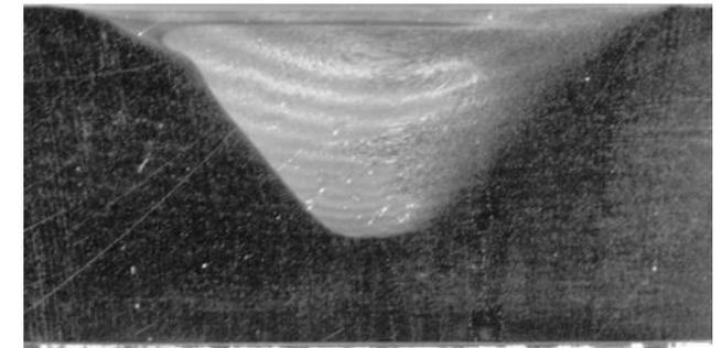
*Friction stir welding and cross section*
