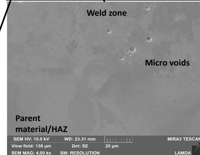
Micro-porosities (~2-10  $\mu\text{m}$ ) were observed in the pool near HAZ.
