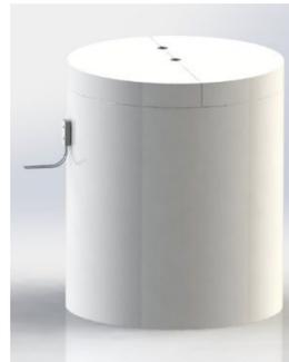
Cylindrical ceramic furnace for heating above container
