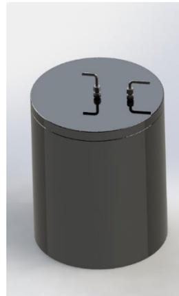
Graphite container with CVD SiC coating on inner and outer surface, ~5kg FLiNaK/batch
