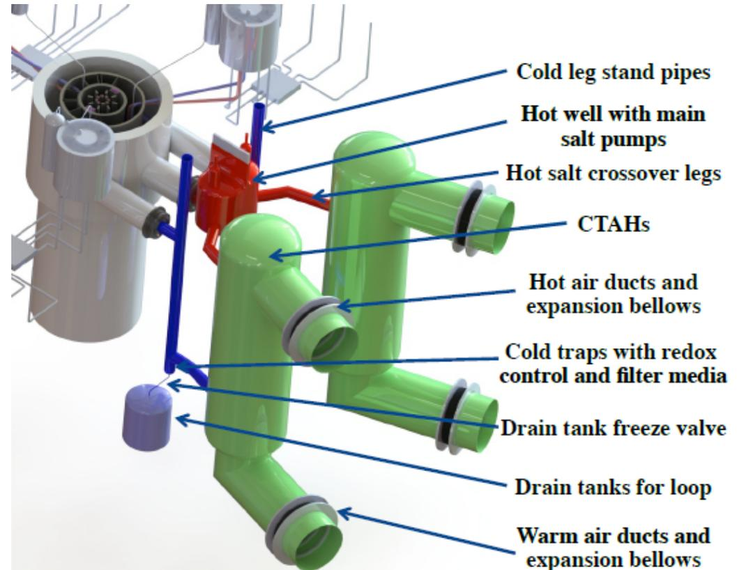
Mk1 PB-FHR, (L) Reactor vessel and cavity, (R) Heat transport system
