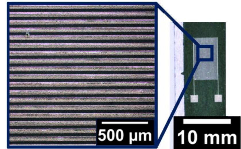
Strain gauge printed at BSU
