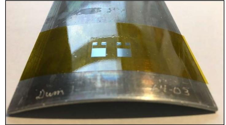
Advanced Manufactured thin film strain gauge on curved ATR fuel plate
