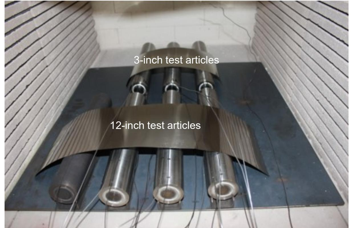
Test articles (small and large) in box furnace
