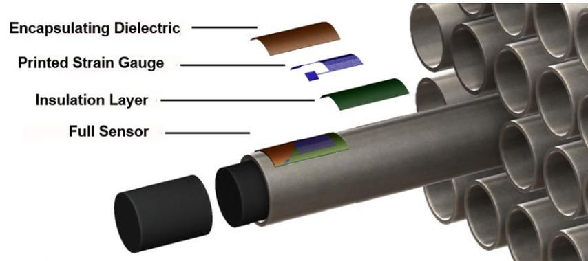
Printed strain gauge design (ASI)
