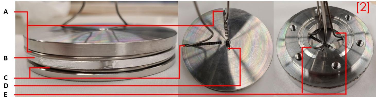
(A) axial guard heater, (B) quartz insulator, (C) main heater, (D) center thermocouple slot, and (E) side thermocouples placed in welded heater assembly cup
