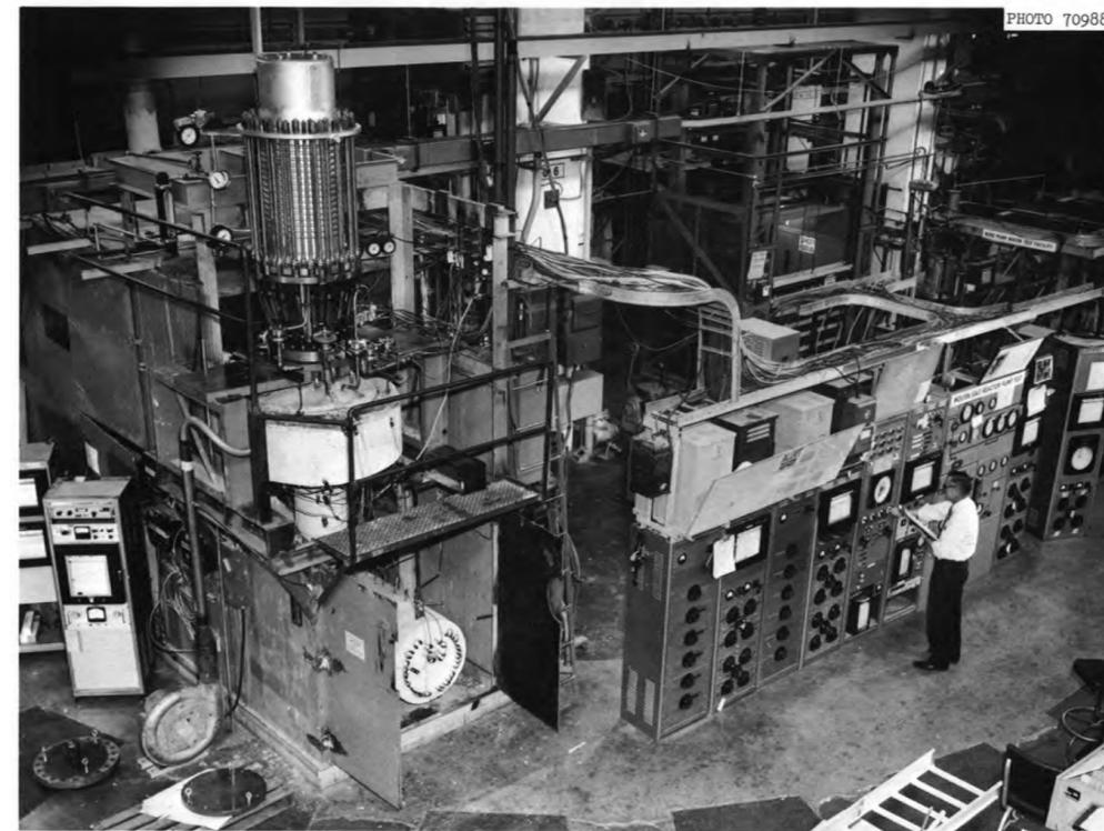
Fig. 4. Photograph of Molten-Salt Pump Test Stand.
