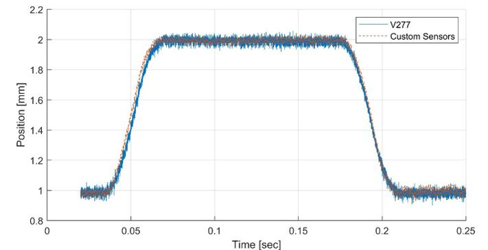
Sensor response at 800 °C and low-temperature commercial position sensor (V277)
