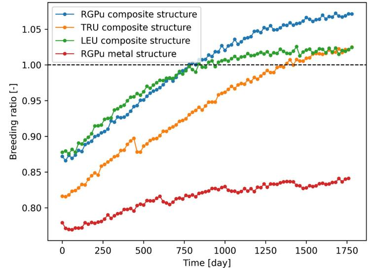
breeding performance for different kick start fuel in composite structure core.
