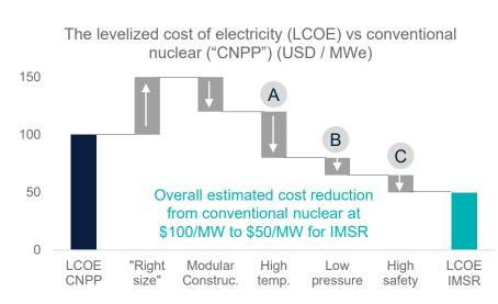
Note: Smaller reactor size drives up cost per MW. This is offset by modular factory production, lower cost, higher temperature and safer operations. Illustrative.
