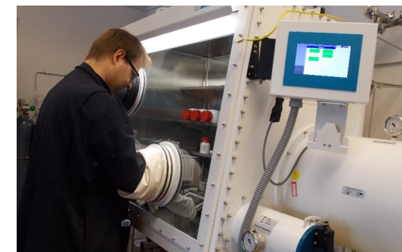
Ar Glovebox ( O_2 < 2 ppm; H_2O < 5 ppm) Handling of non-active and active salts
