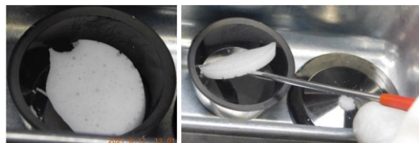
Furnace pre-melt FLiNaK sample LiF-NaF-KF (46.5-11.5-42.0 mol%) Expected T m, Eutectic ~ 454 °C
