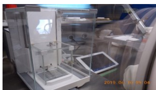
High precision analytical balance in dry argon atmosphere dry-box
