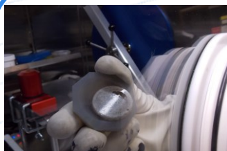
Eutectic salt mixture KCl-MgCl 2 (68–32 mol%)
