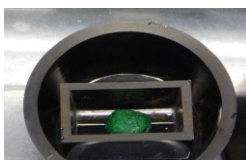
Furnace pre-melt FLiNaK sample LiF-NaF-KF (46.5-11.5-42.0 mol%) Expected T m, Eutectic ~ 454 °C
